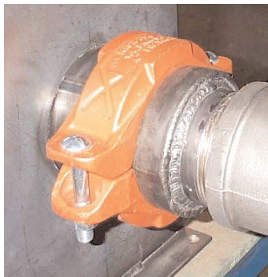
Grooved Couplings for Easy Removal and Cleaning of Heat Exchanger Tubes
